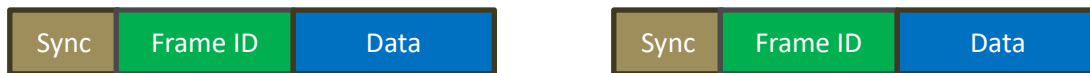
Figure 1 Velocity data structure. The data is composed out of frames, each frame is composed out of three main components the synchronization sequence or the header. The components are schematically shown here, not to scale. The white between the frames indicates that there is pause during the MP data transmission.
